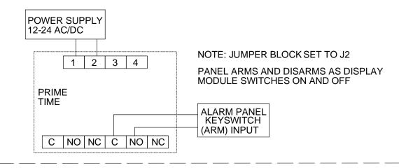
TYPICAL WIRING: TOGGLE MODE WITH FIRST MAN IN ACTIVE USE WITH ELECTRIC LOCK AND DIGITAL KEYPAD FOR TIME CONTROLLED ENTRY SHOWN
